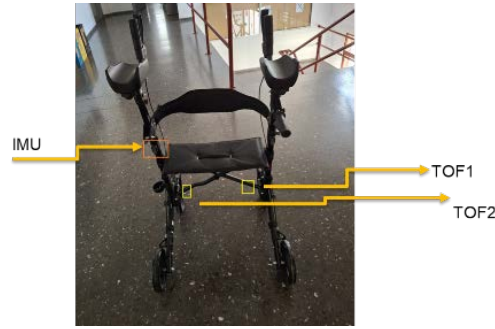
Figure 6. Developed Walker with electronic board integrated in its structure.
