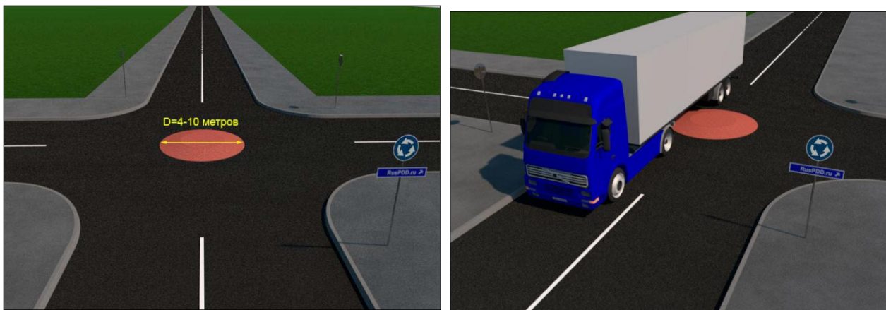
Figure 7. Simple junction with roundabout [3, 12].
