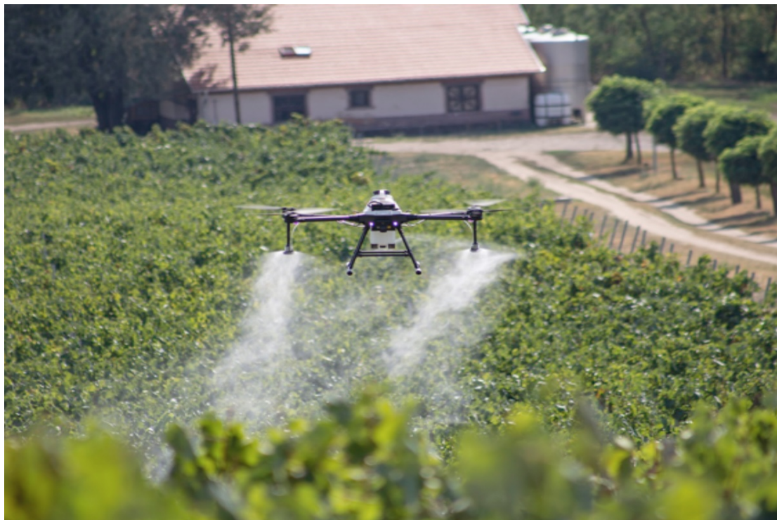
Figure 4. Drone-Based Phytosanitary Treatment System for Precision Protection of Vineyards [26].
