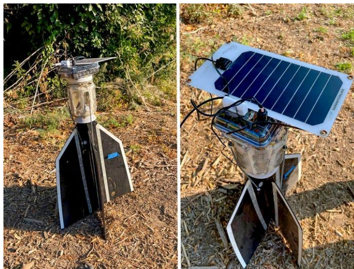
Figure 3. The Pied Piper robot (prototype) for selective pest control in vineyards [15].
