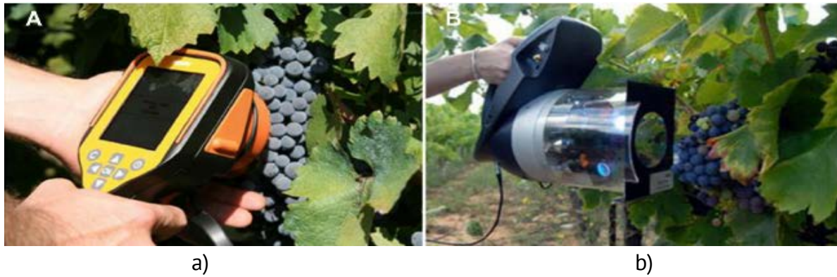
Figure 6. Hand-device Spectron (a) and Multiplex (b) for grape quality proximal quality [32].
