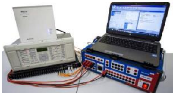
Fig. 5. Apparatus-program test complex based on device CMC 356 of OMICRON company.
